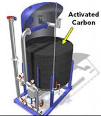
ACTIVATED CARBON FILTER
